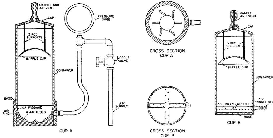
FIG. 3 Air-Jet Dispersion Cups of Apparatus B
