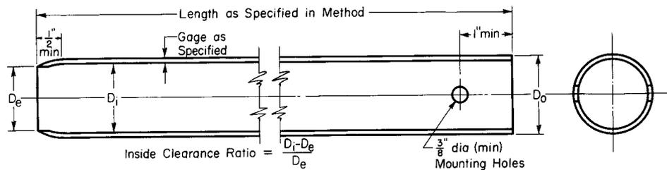
NOTE 1—Minimum of two mounting holes on opposite sides for  $D_o$  smaller than 4 in. (101.6 mm).
